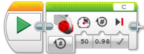
*Note: The Swing Turn could be done using the Move Tank block or the Large Motor block.*
