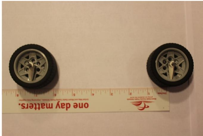
(b) measure the diameter of the wheel and then use the formula  $C=d*\pi$
