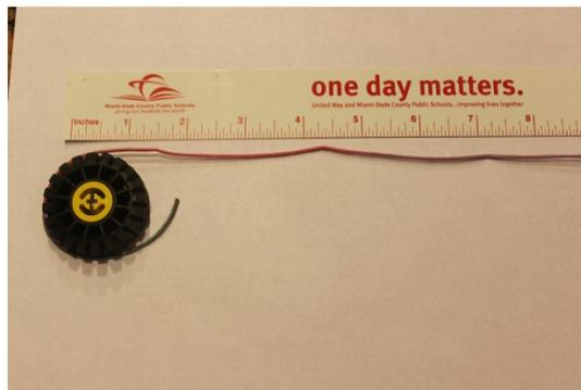
(d) programming the robot to travel one rotation and then measuring the distance traveled
